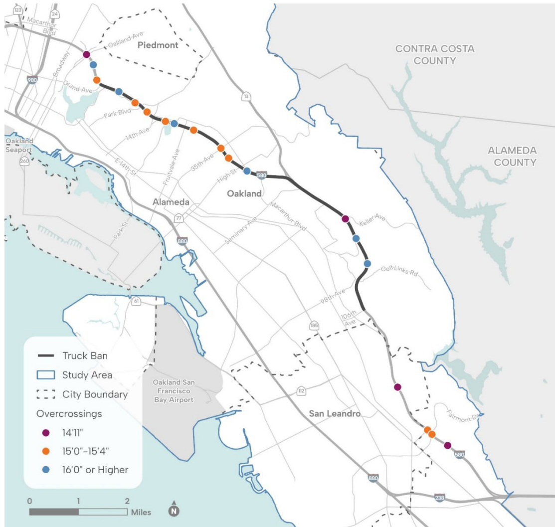
Figure 24: Overcrossing Structure Heights on I-580
